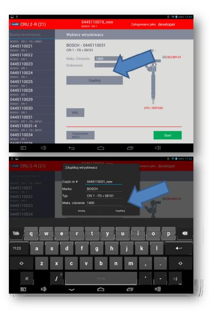
Duplicate test plan, to be edited. Always edit duplicated test plan, to avoid erasing of the original one.
